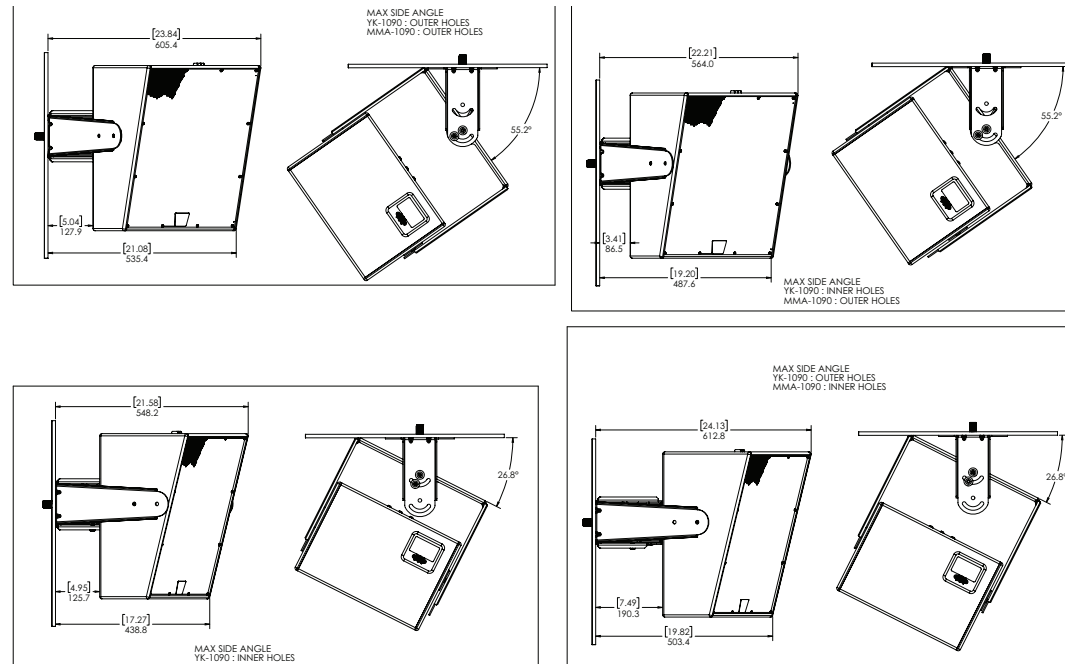
Figure 2-26 CS1090 YK-1090 and MMA-1090 Extended Positions with and Maximum Down Angles [Inches] Millimeters
