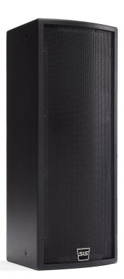
The 8290v2 is a high-quality dual 8", two-way passive design. It serves as a multipurpose system that offers solutions for fill coverage, small-format PA, and stage monitoring. Handles, rigging points, wall bracket mounting points, and a pole socket are provided to serve these purposes.
