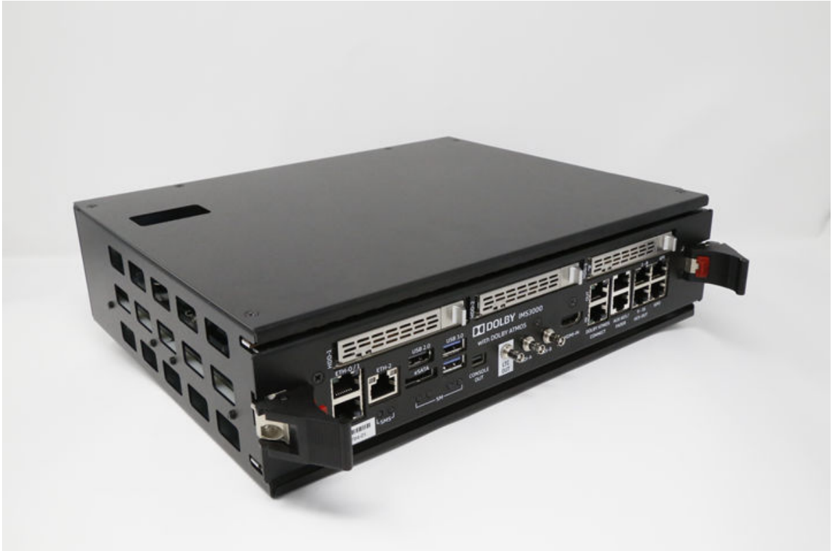
Figure 1: Docking Station with Dolby IMS3000 inserted
