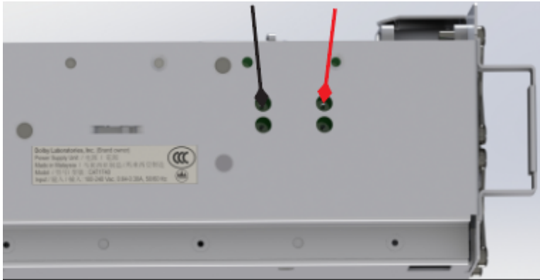
Figure 177: Power supply turned over to test fuse 1 through holes with multimeter probes
