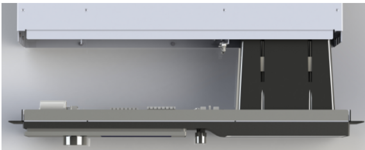
Figure 198: Remove Front Panel from the Chassis
