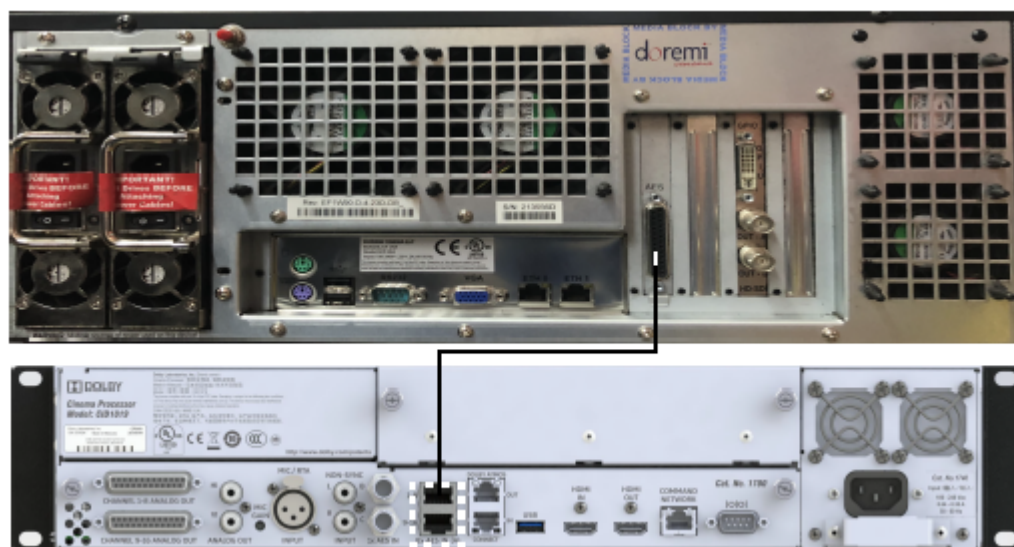
Figure 24: Connecting a Dolby DCP-2K4 to the Dolby CP950
