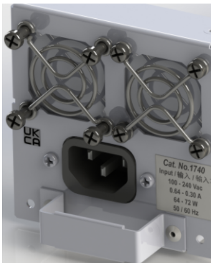
Figure 192: Remove screws from fans
