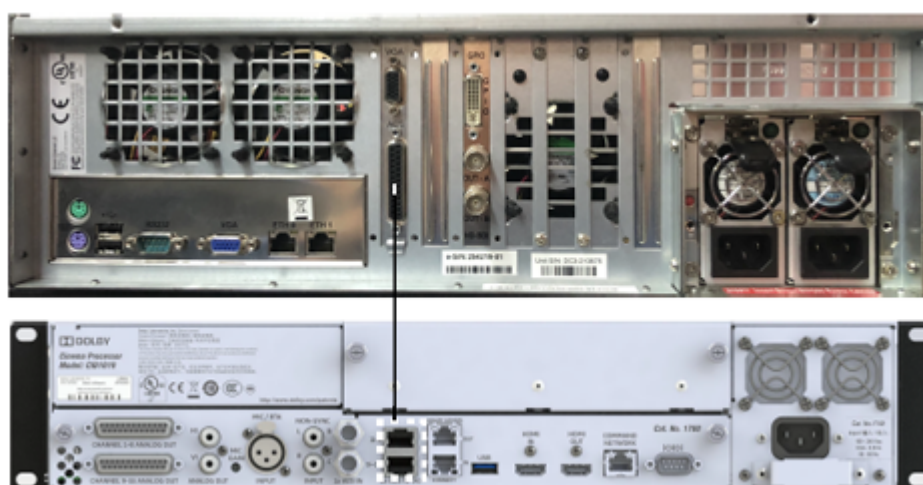
Figure 22: Connecting a Dolby DCP-2000 to a Dolby CP950
