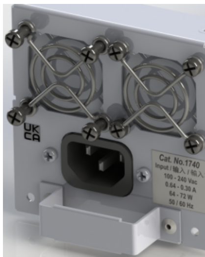
Figure 185: Remove screws from fans
