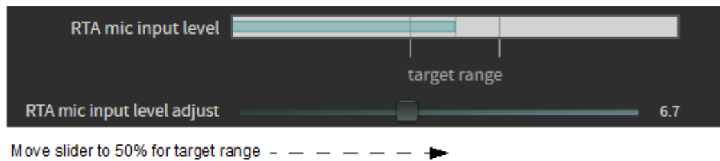
Figure 143: CP950 RTA microphone level adjustment
