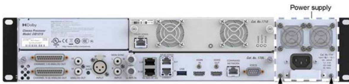
Figure 174: CP950A rear-panel with power supply module and chassis screws
