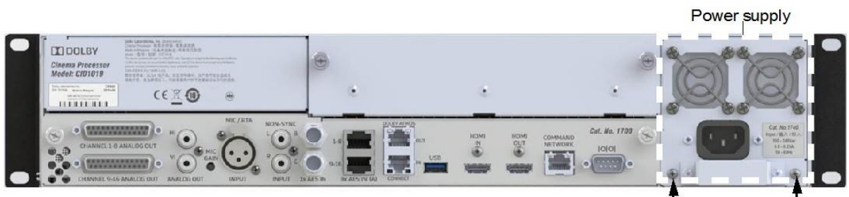
Figure 170: CP950 rear-panel with power supply module and chassis screws
