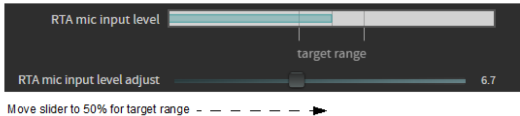
Figure 124: CP950 RTA microphone level adjustment
