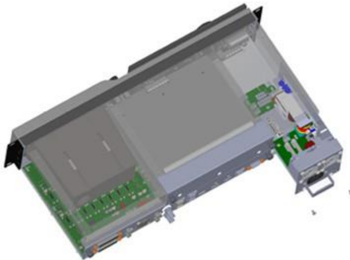
Figure 188: Remove power supply
