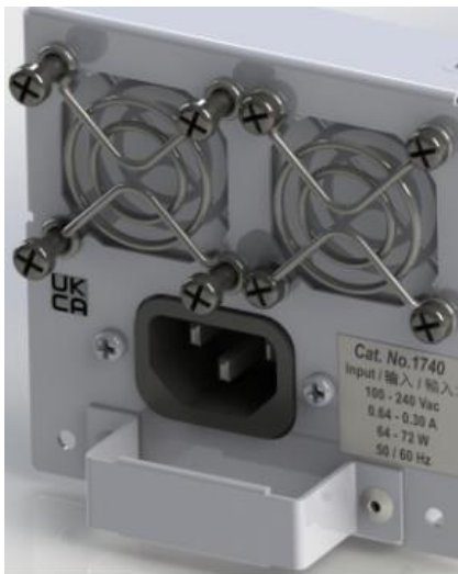
Figure 186: Remove screws from fans
