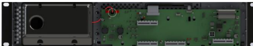
Figure 200: CAT1720 Circuit Board with Booth Monitor Speaker Connection Shown
