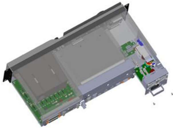
Figure 175: Remove power supply
