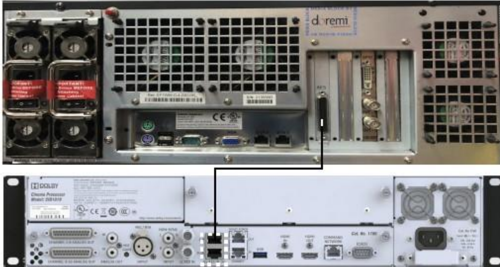
Figure 25: Connecting a Dolby DCP-2K4 to the Dolby CP950A
