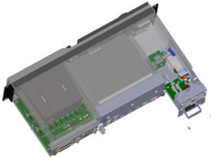
Figure 184: Remove power supply
