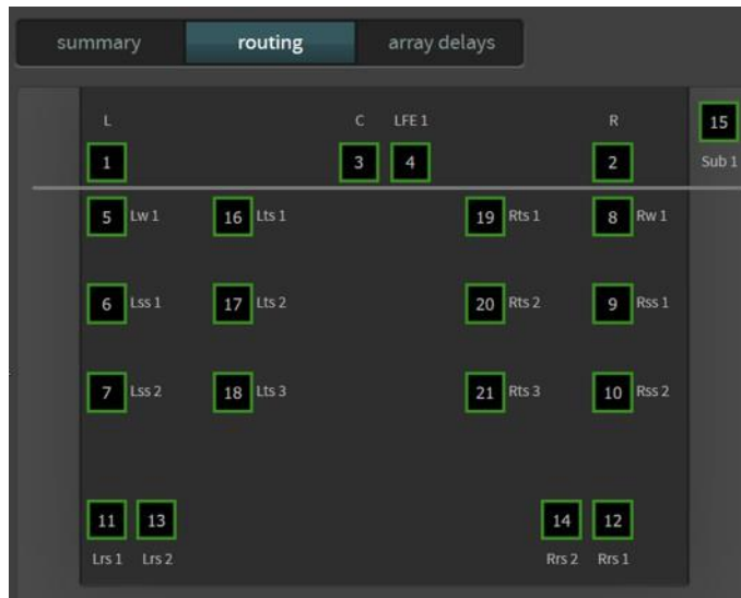
Figure 205: CP850 all digital routing configuration example
