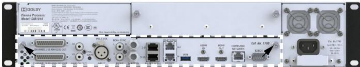
Figure 155: Cat1700 and thumb screws
