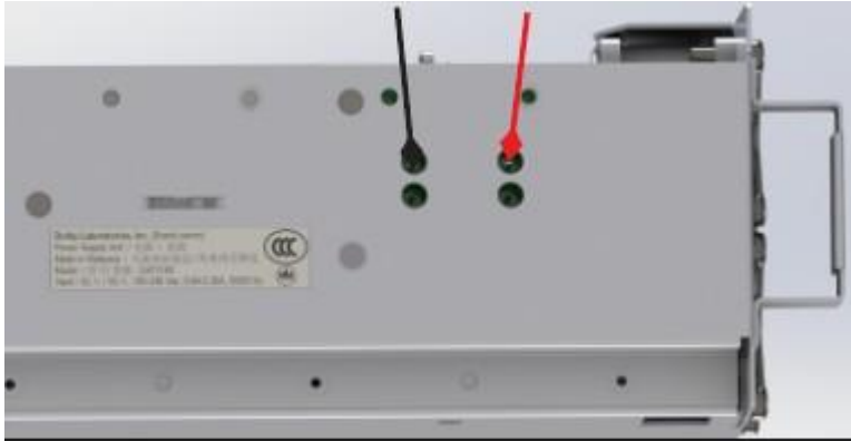
Figure 178: Power supply turned over to test fuse 1 through holes with multimeter probes
