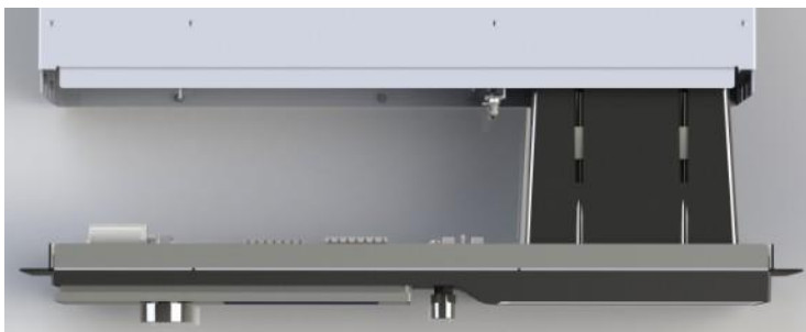
Figure 199: Remove Front Panel from the Chassis
