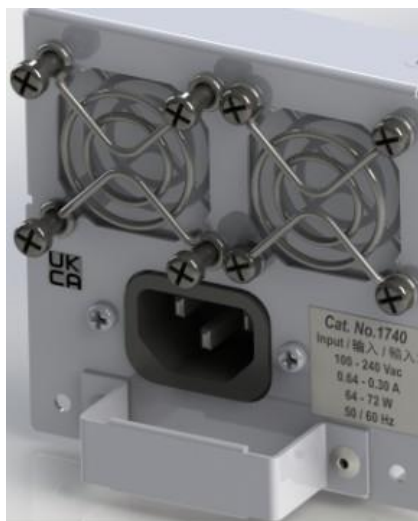
Figure 193: Remove screws from fans
