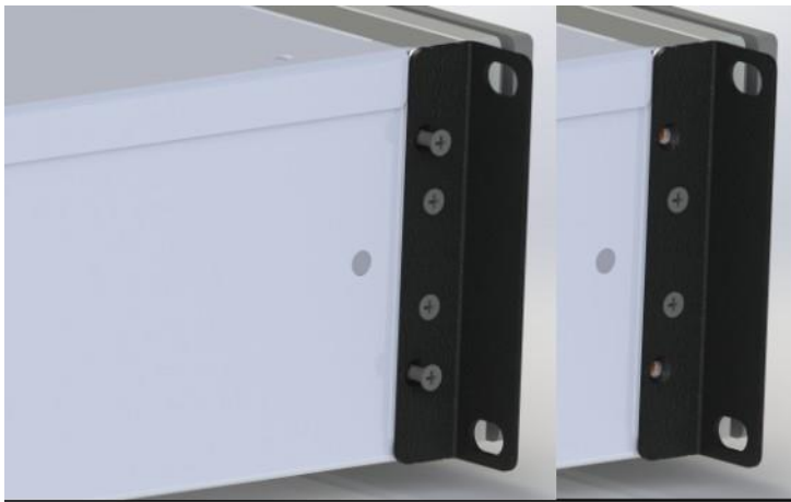
Figure 198: Remove Top and Bottom Screws Behind Rack Ears
