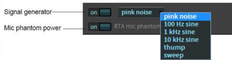
Figure 69: Real-Time Analyzer test-signal generator and microphone phantom Power
