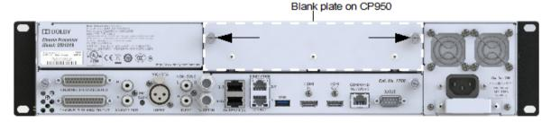
**3.** If the unit is a CP950A, look for the CAT1710 Media Block with two thumbscrews on the rear panel, as shown in the following figure.
