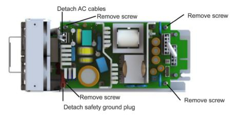
Figure 181: CAT1741 power supply removed from CAT1741 assembly
