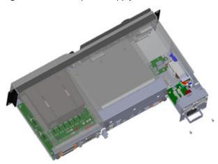
You can see several components on the CAT1741 assembly, as shown in the following figure. The CAT1741 power supply board is mounted on top of the fuses you need to access.
