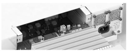
**5.** Remove the three screws that secure the sheet metal fan assembly to the CAT1710 main board (from the bottom side of the CAT1710), as shown in the following figure.
