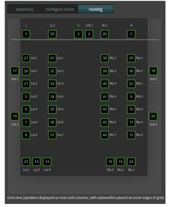
Figure 87: View routing configuration
