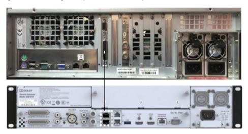
Figure 23: Connecting a Dolby DCP-2000 to a Dolby CP950A
