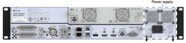
**4.** Use the handle on the power supply to pull the power supply out of the chassis, as shown in the following figure.
