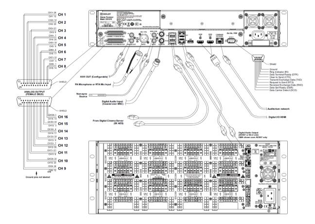
Figure 14: CP950A wiring diagram
