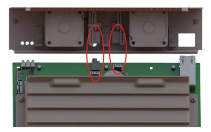
9. Remove the four screws that secure the faulty fan and fan guard, and then remove the fan.
