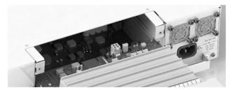
10. Tighten the thumbscrews by rotating them clockwise into the chassis.
