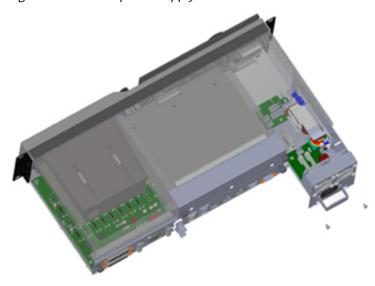
8. Detach the DC power cables (both plugs) from the CAT1741 power supply assembly.
