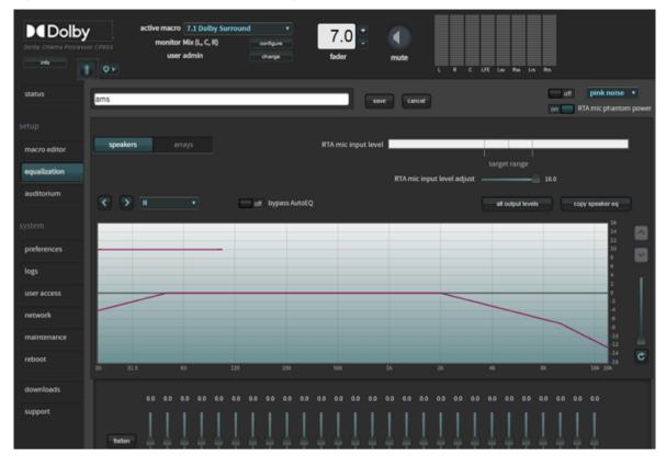
Figure 121: EQ parameters activated for editing
