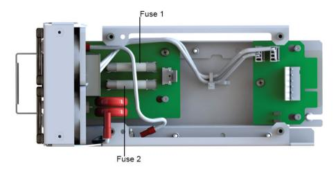
5. You can test the fuses without removing the main power supply card. Turn the power supply over and look for the openings holes in the sheet metal. You can insert multimeter probes through the sheet metal to test the fuses. In the orientation shown in the following figure, the probes are testing fuse 1. Moving to the lower holes allows you to test fuse 2.
