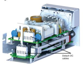
8. Detach the AC power cables (both plugs), detach the safety ground plug, and then remove the four screws that secure the power supply to the CAT1741 assembly. You can now remove the power supply from the sled, as shown in the following figures.
