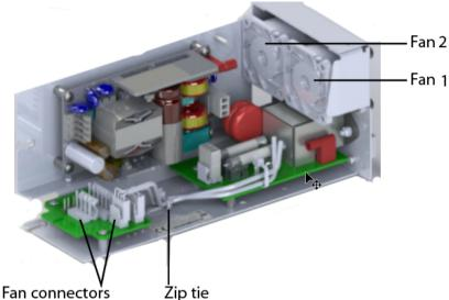
9. If you believe that you found the problem and want to test the fan again, reinstall the power supply in the Dolby CP950, then power up the system. If operation is not restored, you need a new fan. Contact Dolby to order fan part number 8322692. If you are not comfortable replacing fans, you can order a new power supply which is part number CAT1740.
