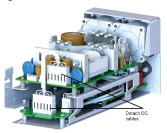
**9.** Detach the AC power cables (both plugs), detach the safety ground plug, and then remove the four screws that secure the power supply to the CAT1741 assembly. You can now remove the power supply board from the sled, as shown in the following figures.
