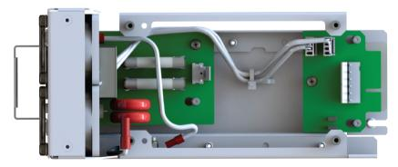
The wires for the fans are plugged into a small circuit board labeled CAT1741-DC. Fan 1 (on the left when viewed from the back of the power supply module) connects to the J2 connector. Fan 2 (on the right) connects to the J3 connector. Reseat the fan connections, then use a flashlight to check if the fan seized
