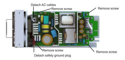
Figure 191: CAT1741 power supply fans and connectors after removing power supply from sled
