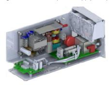
The power moves through the AC input into two fuses on the power supply. Fuse 1 (F1), a 10-amp fuse, is closest to the exposed side of the power supply. Fuse 2 (F2), a 2-amp fuse, is located behind fuse 1. For your convenience, each fuse receptacle supports two fuse sizes, which makes it easier to purchase replacement fuses locally.
