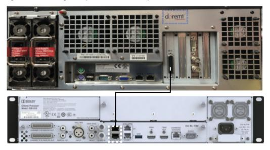
Figure 25: Connecting a Dolby DCP-2K4 to the Dolby CP950A
