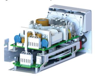
The following figure shows the CAT1741 without the main power supply card installed to help you identify the location of the fuses. You may be able to see that the fuses are labeled on the green circuit board as **F1** and **F2**. Fuse 1 is a 10 A 250 VAC slow blow (time lag) fuse. Fuse 2 is a 2 A 250 VAC slow blow (time lag) fuse.
