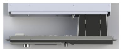
**18.** Check the CAT1720 circuit board for damage. If you had problems with the booth monitor speaker, check the connection on the left side of the board, as shown in the following figure.
