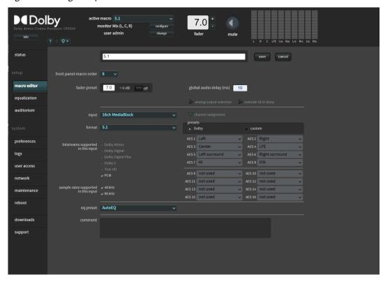
Figure 49: Configure input source for 16ch MediaBlock
