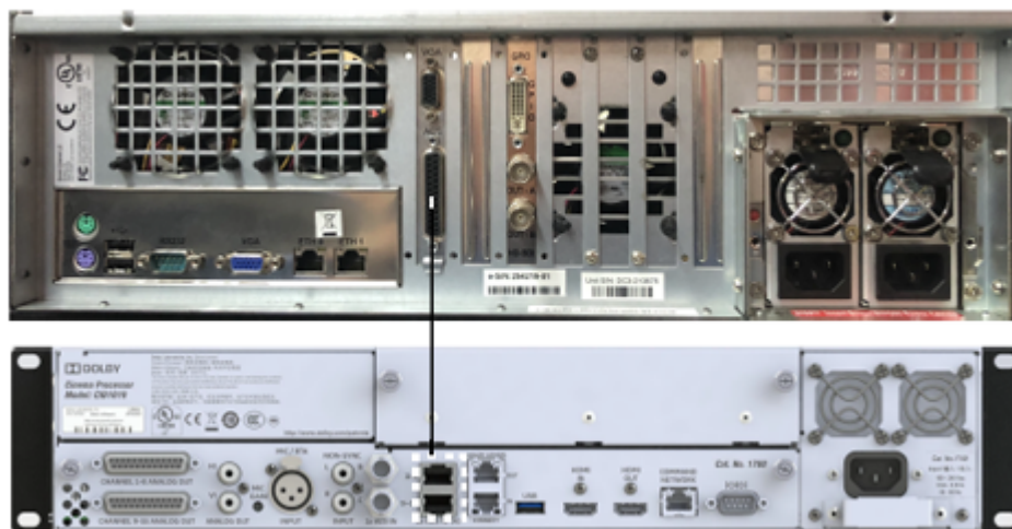
Figure 23: Connecting a Dolby DCP-2000 to a Dolby CP950A
