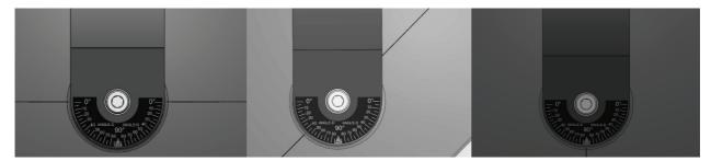
Figure 2-3 Angle D at 0, 45, and 90 Degrees Using Speaker Body Parting Line as Indicator
