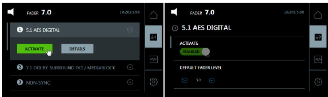
2. Press **ACTIVATE** to enable the selected macro. Press **DETAILS** to view the parameters for the selected macro. You can set the default fader level when the macro is **ENABLED**.
