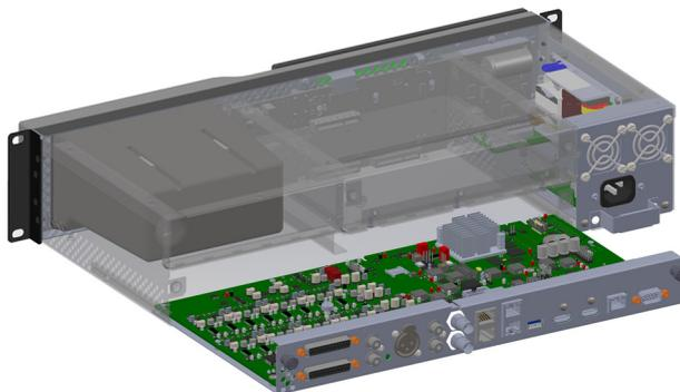
5. Inspect the CAT1700 main board for signs of damage to its components or the edge connector that plugs into the CAT1720 front-panel board. If there is damage, you may need to replace the CAT1700 or CAT1720.
