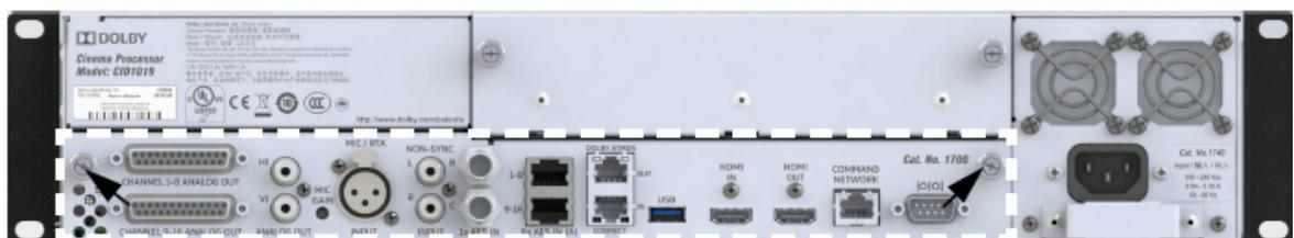
3. Unscrew the thumbscrews in a counter-clockwise direction. These screws are captured in the chassis and do not come out completely.
