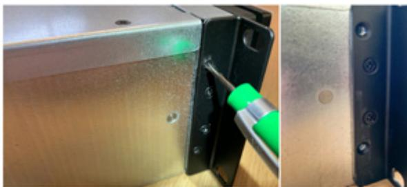
14. Pull on the rack ears to remove the front panel straight out of the chassis.
