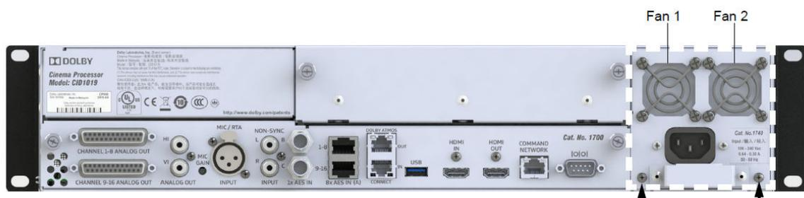
4. Use a small Phillips screwdriver to remove the two screws that secure the power supply to the chassis.
