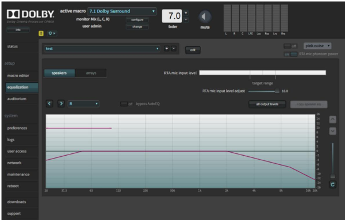
**Test signal generator and microphone phantom power**
