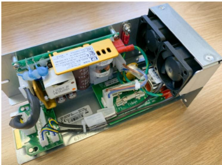
The power moves through the AC input into two fuses on the power supply. Fuse 1 (F1), a 10-amp fuse, is closest to the exposed side of the power supply. Fuse 2 (F2), a 2-amp fuse, is located behind fuse 1. For your convenience, each fuse receptacle supports two fuse sizes, which makes it easier to purchase replacement fuses locally.
