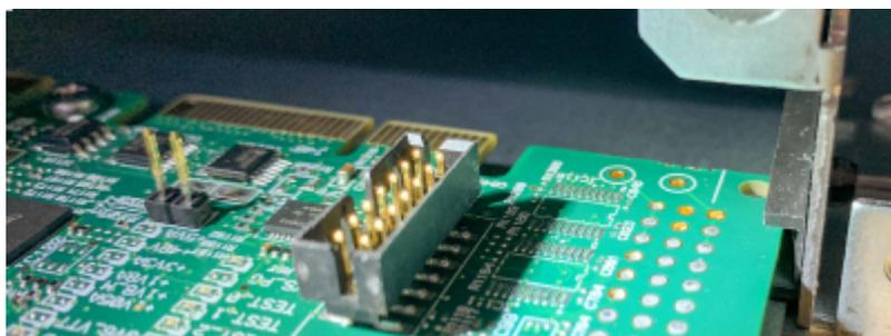
7. Push the CAT1700 carefully into its final position using the guide rails, and then use the thumbscrews to secure the board to the Dolby CP950 chassis.
