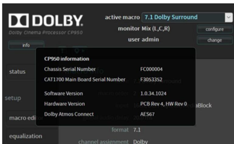
If you need an RMA for a faulty part, the **info** button is a good resource where you can find the CP950 chassis serial number. This is the main serial number for the unit and is required for all RMAs. The CAT1700 main board contains all of the inputs and outputs and controls audio processing.
