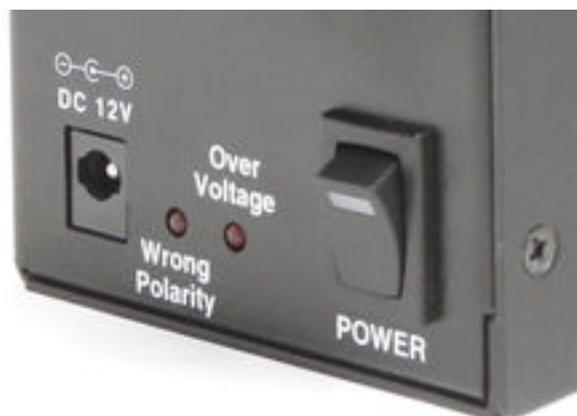
If you connect a power supply and the wiring has reversed polarity (tip negative), the **Wrong Polarity** LED will illuminate. To fix this issue, change the polarity of the wiring to be tip positive.
