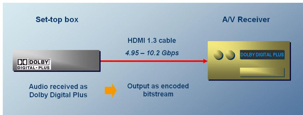
**Figure 2b:** The HDMI Connection on a Set-Top Box Allows a Full Dolby Digital Plus Stream to Be Transmitted Directly
