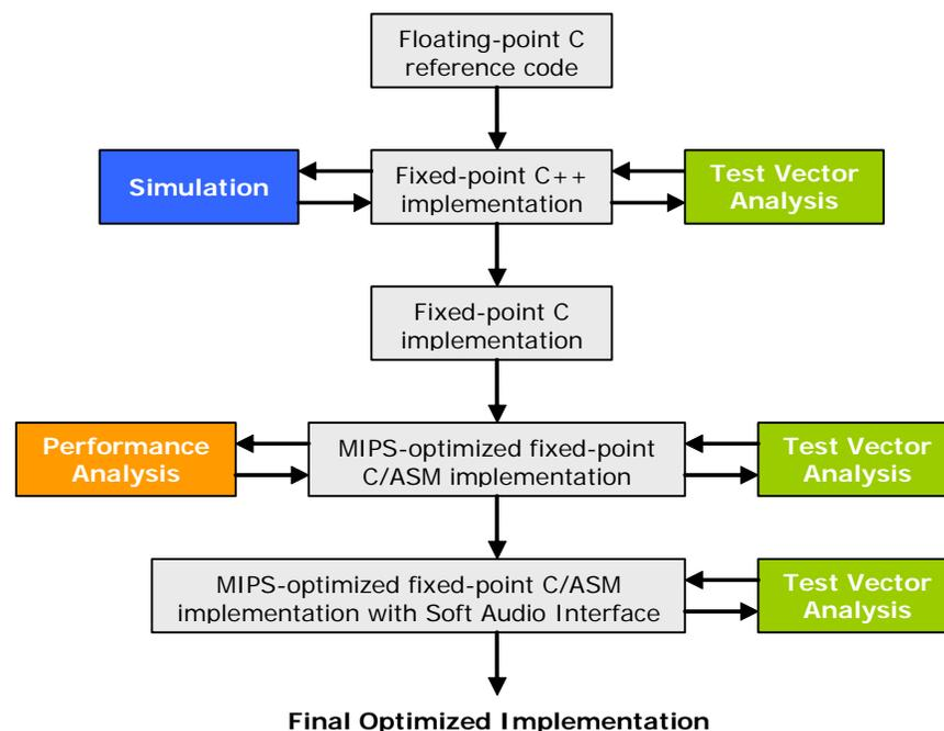
**Figure 4:** Converting Floating-Point Dolby Code to Highly Optimized Fixed-Point MIPS32 Code
