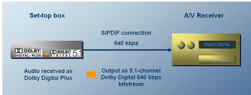
**Figure 2a:** The S/PDIF Connection from STB or Optical Disc Player to an A/V Receiver
